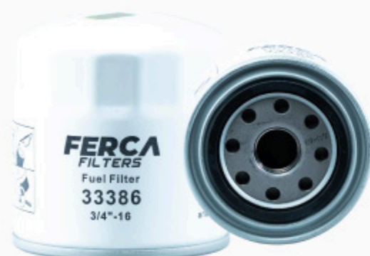
COD. 33386 Rosca: 3/4"-16 CHEVROLET NPR 3.9 / NPR 66L NPR 71L / FVR / FVR 23G / FVR 33K Altura: 90mm Diametro exterior: 80,5mm
